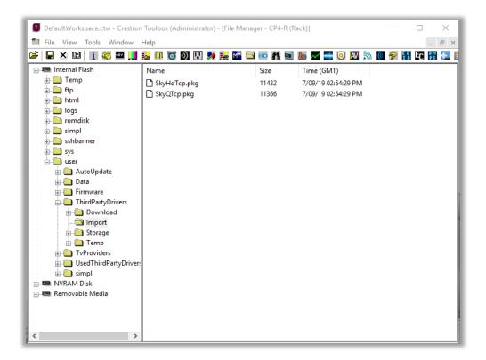
Once the files are copied, the Crestron Home system will automatically import the drivers and rebuild the driver list in the Crestron Home configuration system. This may take a few minutes and, once imported, the driver package files will disappear from the "Import" directory, though you may need to refresh your file system window to see this.
